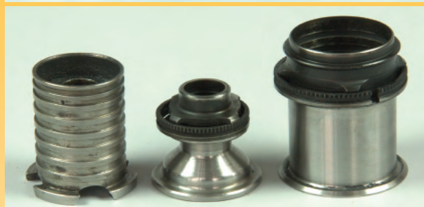
Above: Evolution of Beretta's pistons: (l. to r.): 391, A400, Xtrema2.
