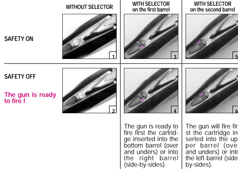
**WARNING:** Do not attempt to make repairs to any firearm without proper knowledge or training. Do not alter parts or use substitute parts not made by Beretta. Any alterations or adjustments that may be necessary to the operating mechanism should be performed by the Manufacturer or by its Local Official Distributor.
